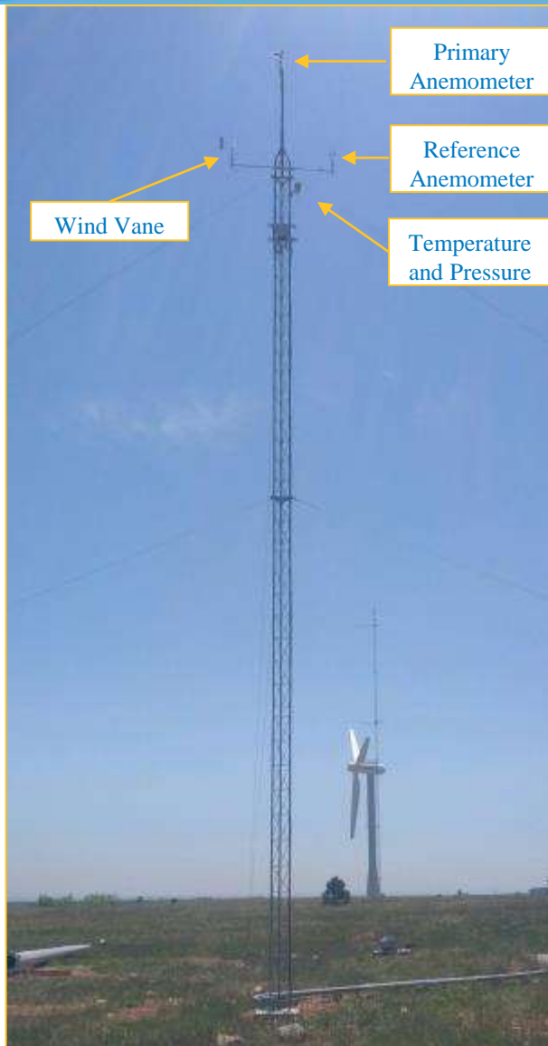
Met tower and instrumentation used for field test campaign (Photo by Scott Dana, NREL)
