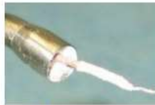
Figure 2: sonotrode ripped out
