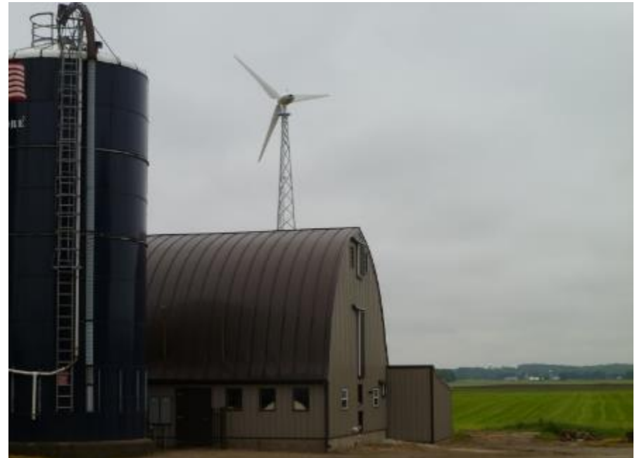
Endurance E3120 turbine; 50-kW turbine, Appleton, Wisconsin Photo from Kettle View Renewable Energy, LLC, NREL 28428
